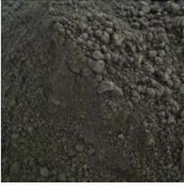
**Ore concentrates can be very sticky and cohesive, particularly when wet. Poor bin and feeder design will lead to permanent, chronic bridging and plugging when handling particularly difficult flowing materials.**
