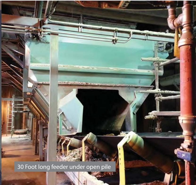
30 Foot long feeder under open pile
